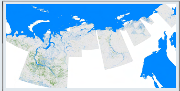
Mosaic of Envisat ASAR derived wetland classification maps of northern Russia in 2007, showing maximum open water in blue and permanently high saturated areas in green.
