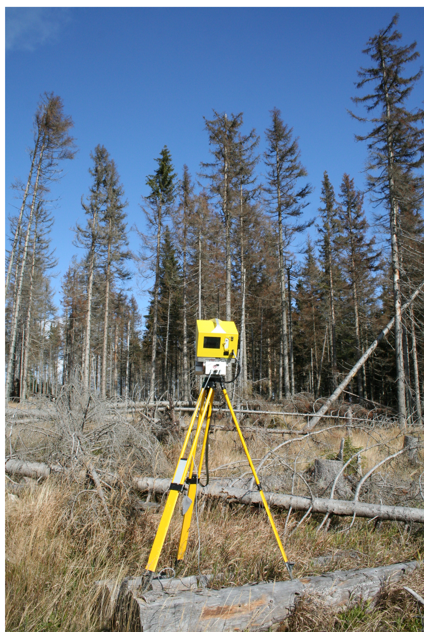
Figure 8 Terrestrial laser scanner OPTECH Ilris-36D.
